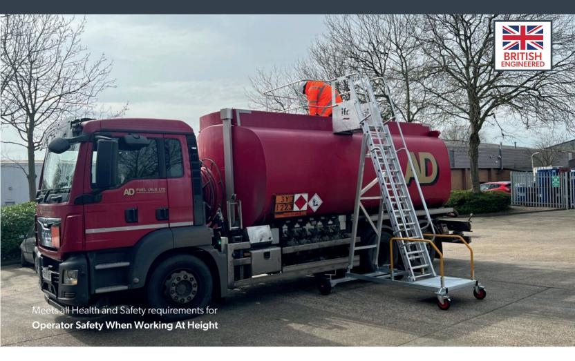
Our newly redesigned TopTank system is one of our mobile fall prevention solutions. It allows you to safely access the tops of road and rail tankers, and ISO containers without the need for fixed gantries, fall arrest harnesses or relying on inbuilt tanker railings.
