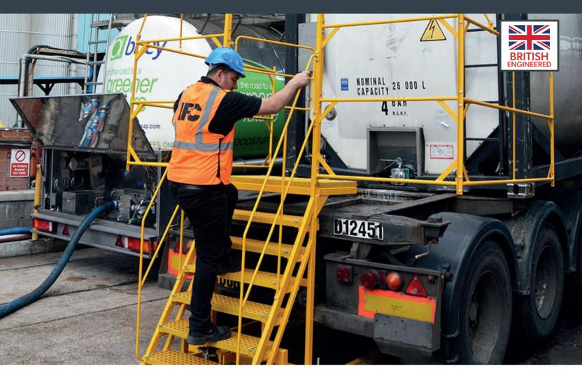
Our LowTank mobile tank access ladders are designed to offer safe and easy access onto the back of ISO tank trucks. It has an integral three-rail safety cage that provides a safe working area while on the truck bed and helps prevent falls from height associated with ISO tank operations.
