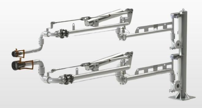
The BLA-803 duplex or double bottom loading /unloading station reduces the risk of spills or accidents while loading and unloading bulk liquid road and rail tanks. These highly engineered arms are designed for applications where a liquid and vapour line are required for bottom loading or unloading operations. These arms can be used for cryogenic products as well as a range of hazardous and specialist liquids.
