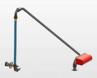
The BLA-100 is a fixed length boom type arm with a base swivel for horizontal movement and an optional vertical swivel and spring balance for vertical movement. It is typically used for railway and heavy plant refuelling where an extended reach is required from the fixed filling system. It can be used for fuels and chemicals.
